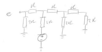
0.5 V would appear on the output [1]. A very good attempt simplifying the R2R ladder circuit to prove the output would be 0.5 V [4].
