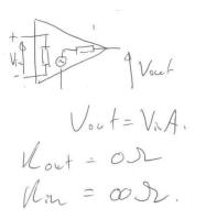
d. \*Marks for correctly drawn non-inverting op-amp [3]
